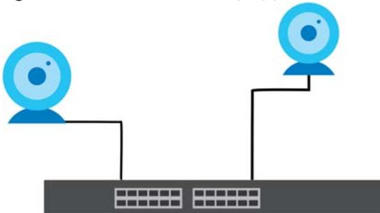
**The PD may stop responding to the Switch's detection over ping or LLDP during firmware upgrade. Disable the Auto PD Recovery function to prevent damage to the PD caused by a power cutoff during firmware upgrade.**
