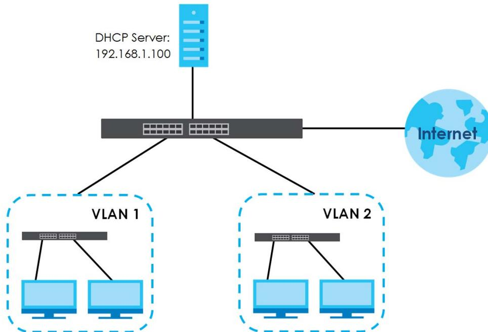
Configure the **DHCP Relay** screen as shown. Make sure you select a DHCP option 82 profile (**default1** in this example) to set the Switch to send additional information (such as the VLAN ID) together with the DHCP requests to the DHCP server. This allows the DHCP server to assign the appropriate IP address according to the VLAN ID.
