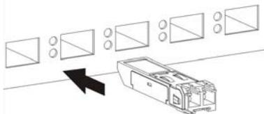
**Figure 20** Connecting the Fiber Cables
