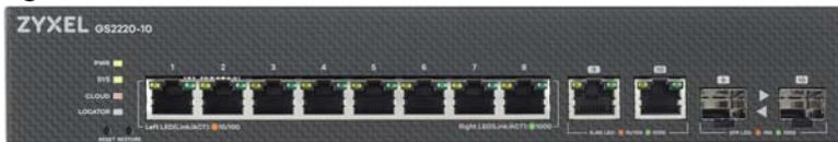
Figure 13 Front Panel: GS2220-10HP
