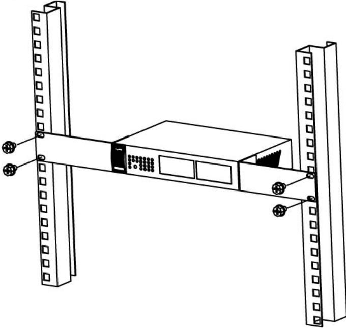
**Figure 11** Mounting the Switch on a Rack
