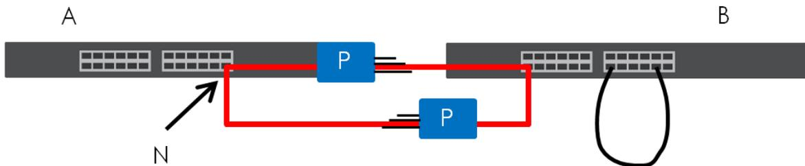
The Switch also shuts down port N if the probe packet returns to switch A on any other port. In other words loop guard also protects against standard network loops.
