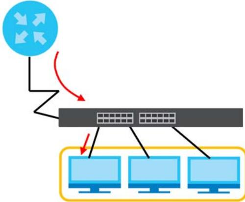
Figure 127 Static Multicast Forwarding to Multiple Ports
