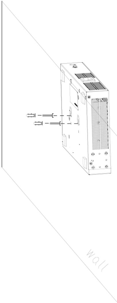
**WARNING!** The Switch should be wall-mounted horizontally, and make sure the front panel is facing down. The Switch's side panels with ventilation slots should not be facing up or down as this position is less safe.
